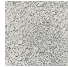
CRUSHED MATERIAL: crushed stone fraction mixture ranging from 0 to 16 mm
