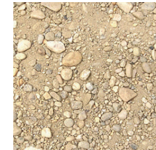
ROUND GRAIN MATERIAL: river gravel with fractions ranging from 0 to 32 mm
